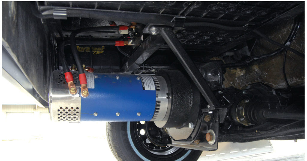
The motor for this kit (Model # FB1-4001) is also made by Advanced DC Motors, the best known name in the industry. The motor dimensions are 9.1 inch diameter 15.5 inches long, and is rated at 144 Volts DC. Rain and water won't hurt the motor unless it is totally submersed. Though it isn't a bad idea to protect it against rocks and dust with some type of cover underneath, it's important to make sure there is some air flow to the motor to keep it from overheating.
